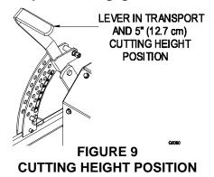
d) Insert height adjustment pin into hole corresponding to desired cutting height and install hairpin cotter. See decal on the side of deck lift plate.
